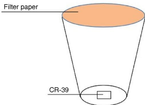
**Figure 2. Schematic diagram of the geometry of the CR-39 radon detector used**
